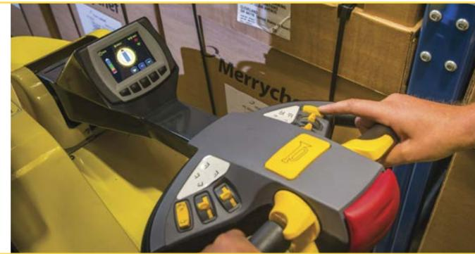
Incorporating the benefits of AC technology in its traction, pump and steering motors, the Combi-WR has a lift height that can be tailored to your application with load capacities up to 1,450kg.
