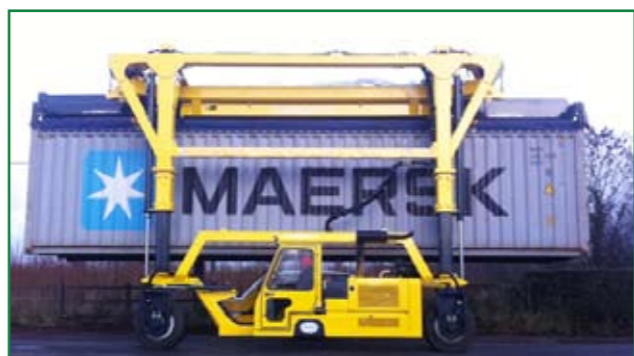
The retracted telescopic frame allows entry under low doorways, while the extended telescopic frame allows double stacking.
