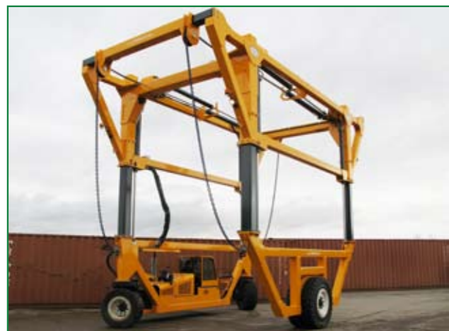
The retracted telescopic frame allows entry under low doorways, while the extended telescopic frame allows double stacking.
