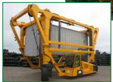
◀ Same Unit can lift 20', 30', 40', 45' Containers
