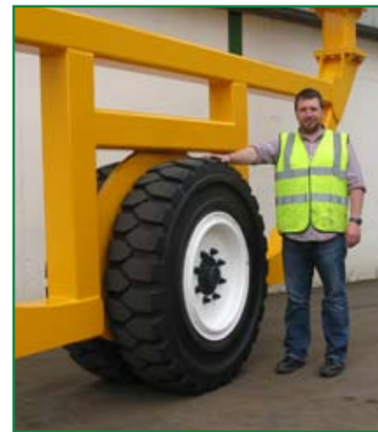
▲ Large Tyres for Low Ground Pressure
