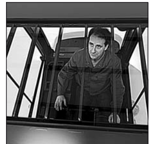
Clear-view overhead guard
