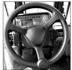
Fully hydrostatic steering
